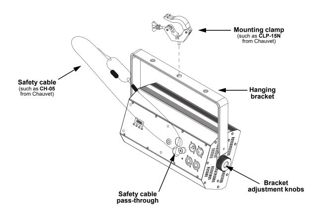
To prevent accidental loosening when using a single mounting clamp, be sure to use a clamp with a captive bolt.
