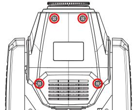
3. Remove 4 screws with a Phillips-head screwdriver to remove the cover.
