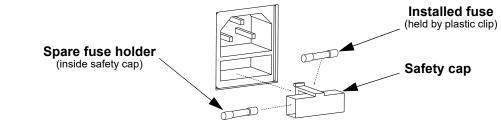
Disconnect the product from the power outlet before replacing the fuse.
