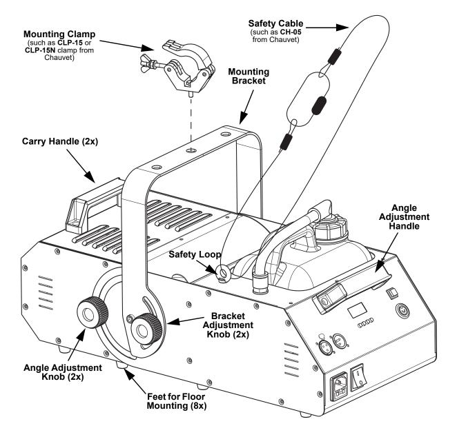
When using only one mounting clamp with this fixture, you must use a clamp with a captive bolt to prevent accidental loosening.
